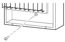
Figure 11 - Installing Bottom Mounting Screw
